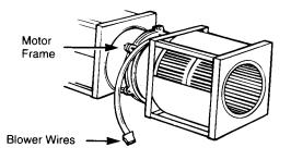
Caution To avoid product failure, do not pull, stretch, or pinch blower wiring. 8. Replace blower plate using 5 screws.
